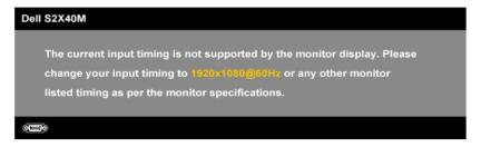
This means that the monitor cannot synchronize with the signal that it is receiving from the computer. See <u>Monitor Specifications</u> for the horizontal and vertical frequency ranges addressable by this monitor. Recommended mode is 1,920 x 1,080.
