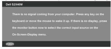
If VGA or DVI cable is not connected, a floating dialog box as shown below appears. The monitor will enter Power Save Mode in 5 minutes if left at this state.
