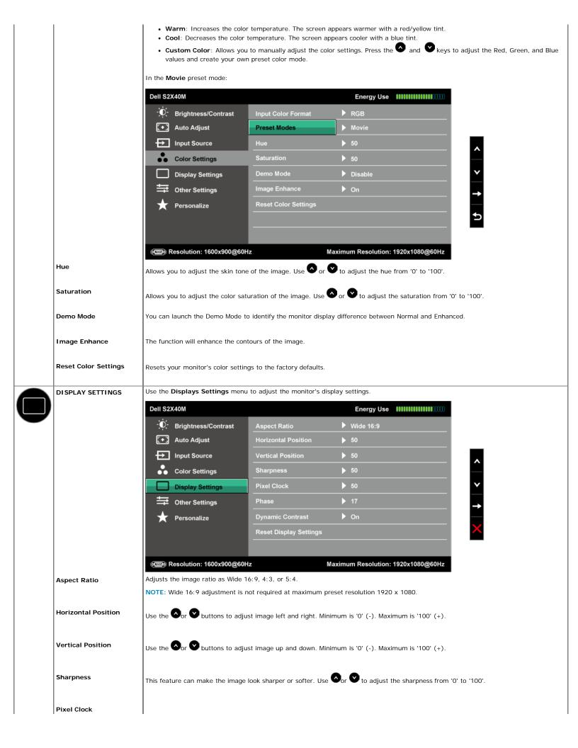
The Phase and Pixel Clock adjustments allow you to adjust your monitor to your preference. Use or buttons to adjust for best image quality.
