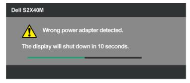
To avoid damage to the unit, user is strongly advised to use the original power adapter that comes packaged together with the monitor.
