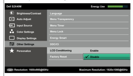
If an image appears to be stuck on the monitor, select **LCD Conditioning** to help eliminate any image retention. Using the LCD Conditioning feature may take some time. LCD Conditioning feature cannot remove severe cases of image retention or burn-in. **NOTE**: Use LCD Conditioning only when you experience a problem with image retention.
